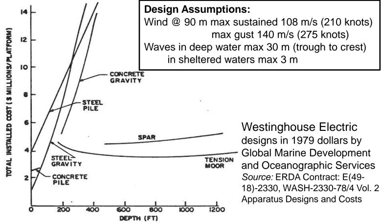
Severe wind and wave design drivers for ocean applications favor shallow sheltered water using gravity and driven pile platform designs
